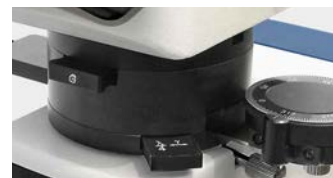
Bertrand lens, \lambda Slip, 360° rotatable analyser (removable)
