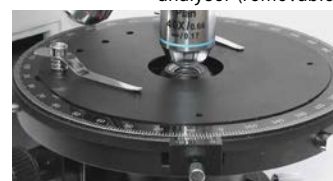
Center-adjustable and turnable polarisation stage
